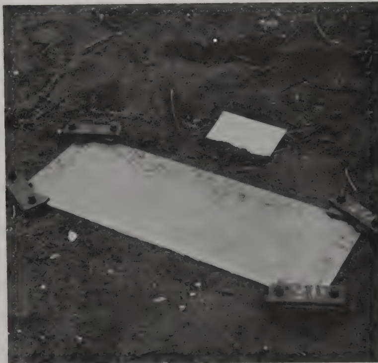
FIG 12 MODEL PANEL IN SURFACE BEFORE FIRING.
